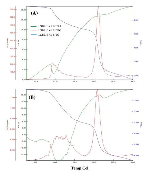
Fig. 4. TG and DTG curves of the produced levan catalyzed by (A) Lsbl-bk1 and (B) Lsbl-bk2. Blue, red, and green lines show TG, DTG, and DTA curves, respectively.
