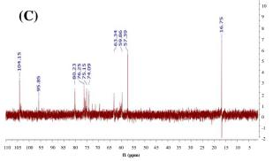
**Fig. 2.** Analysis of the produced levan catalyzed by Lsbl-bk1: (A) FTIR spectrum of levan (black line) compared with levan standard from *E. herbicola* (red line), (B) levan <sup>1</sup>H-NMR spectrum, and (C) levan <sup>13</sup>C-NMR spectrum.
