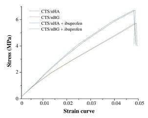
Fig. 5. Stress vs. strain curve of ibuprofen-loaded and -unloaded scaffolds.
