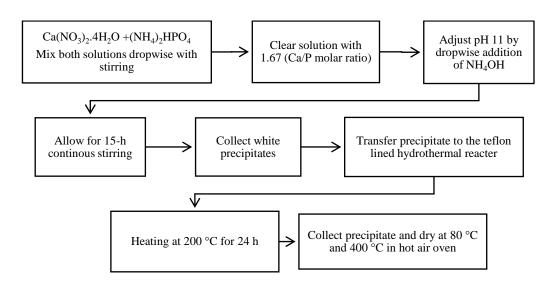
Fig. 1. Hydroxyapatite nanoparticles (nHA) synthesis using hydrothermal method.
