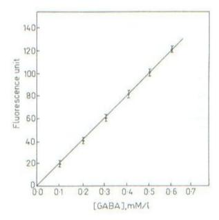
**Fig. 1.** Calibration of GABA. Different GABA concentrations have been subjected to GABA assay test and NADPH enzymatic cycling method. The fluorescence emission has been measured at 455 nm. Each point is the average of two determinations. For experimental details see the material and method section.
