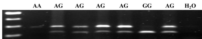
**Fig. 2.** Genotype analysis for the *MTHFD1* gene. The wild type (G) allele was digested with restriction endonuclease *MspI*. H<sub>2</sub>O is a negative control reaction without DNA.
