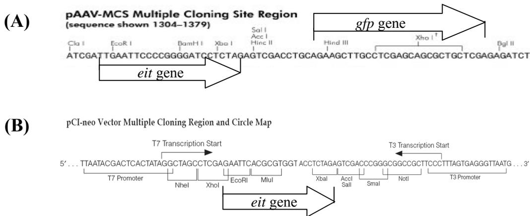
**Fig. 1.** Map of pAAV-MCS and pCI-neo vectors. In the pAAV-MCS, *gfp* gene was cloned between *Bgl*III and *Hind*III and the *eit* gene was inserted between *Eco*RI and *Sal*I restriction sites (A). In the pCI-neo vector, the *eit* gene was inserted between *Eco*RI and *Sal*I restriction enzymes (B).
