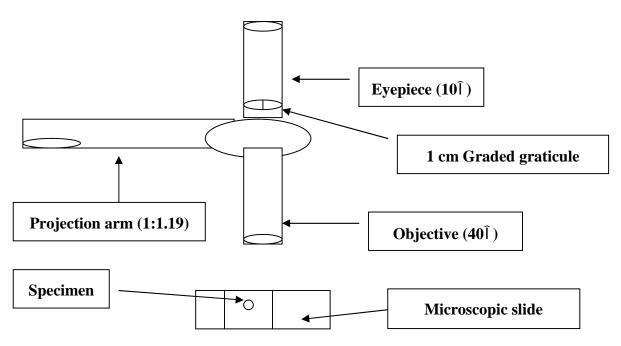
**Fig. 1.** A simplified diagrammatic representation of the microscopic arrangement for measurement of the thickness of rat aorta samples. Note that the magnification for the sample projected to the eye piece is  $400\times$ , which is reduced by the projection arm by a factor of 1: 1.19, providing a final magnification at the projection end  $336\times$  that of the actual thickness of the sample.
