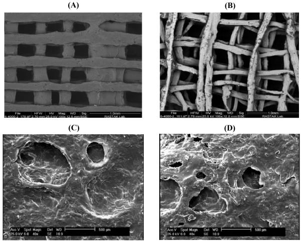
**Fig. 4.** Electron microscopy images of the prepared films. SEM image for (A) drug-loaded films (magnification of 1.00 mm); (B) drug-unloaded films (magnification of 1.00 mm); (C) drug-loaded films (magnification of 500 μm); (D) films without drug (magnification of 500 μm).
