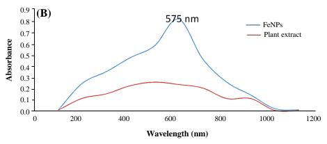
Fig. 2. (A) Visual inspection of color change for the formation of FeONPs; (B) UV-Vis spectroscopy of FeONPs and plant extract.
