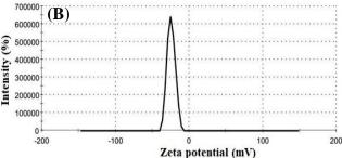
Fig. 2. Zeta potential of SFNPs before (A) and after (B) drug loading.
