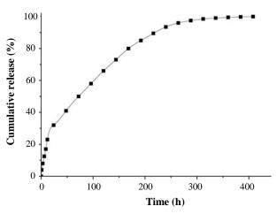
**Fig. 5.** Release profile of simvastatin from SFNPs at pH 7.4. The drug had a slow release rate from the NPs due to strong hydrophobic interactions between the drug and SFNPs.
