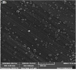
**Fig. 3.** SEM images of SFNPs before (A) and after (B) drug loading. The NPs had spherical morphology with uniform size distribution (magnification: 500 nm).
