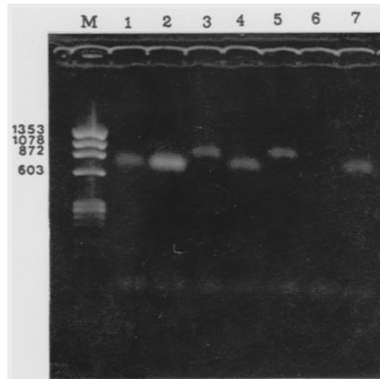
**Fig. 2.** Gel electrophoresis of PCR product isolated from control strains and fowl feces. Lane M, Molecular weight marker; lane 1-3: Control strains; lane 1, *C. jejuni* Lior 1; lane 2, *C. jejuni* Lior 2; lane 3, *C. coli* Lior 8; lane 4 and 7, *C. jejuni* isolated from fowl feces; lane 5, *C. coli* isolated from fowl feces; lane 6, Non-*Campylobacter jejuni* and *coli* specimen.
