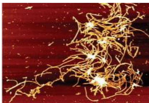
Fig. 1. Atomic force microscopy of A \beta 1-40 peptides after being dissolved in PBS and incubated for one week. The Figure shows many fibril clusters from A \beta 1-40 peptides aggregation. Scan size = 500 \times 500 nm.
