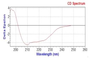
**Fig. 6.** Results of CD analysis by CDNN software (Circular Dichroism analysis using Neural Networks). Nucleoprotein (0.3 mg/mL) in 50 mM of  $Na_3PO_4$ , pH 7.5 was tested in the CD system. Spectra were recorded in 180-260 nm on a Circular Dichroism Spectrometer Model-215, Aviv, USA at a scan speed of 1 nm/sec.
