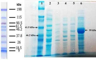
**Fig. 3.** Washing steps of inclusion bodies. Lane 1, protein marker; lane 2, supernatant of second wash with lysis buffer; lane 3, supernatant of second wash with Tris EDTA Tween-20; lane 4, supernatant of second wash with Tris EDTA NaCl; lane 5, supernatant of second wash with Tris EDTA urea; lane 6, solubilized protein in solubilization buffer.
