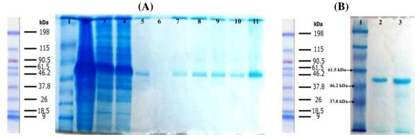
**Fig. 4.** Protein purification on AbCA-AbC column. (A) lane1, protein marker; lane 2, extracted protein from cultured media before washing steps; lanes 3 and 4, inclusion bodies after washing steps; lanes 5 and 6, washing the column with refolding buffers; lanes 7-11, protein eluted from column with the elution buffer. (B) Lane 1, protein marker; lane 2 purified protein; lane 3 concentrated protein using Amicon column.
