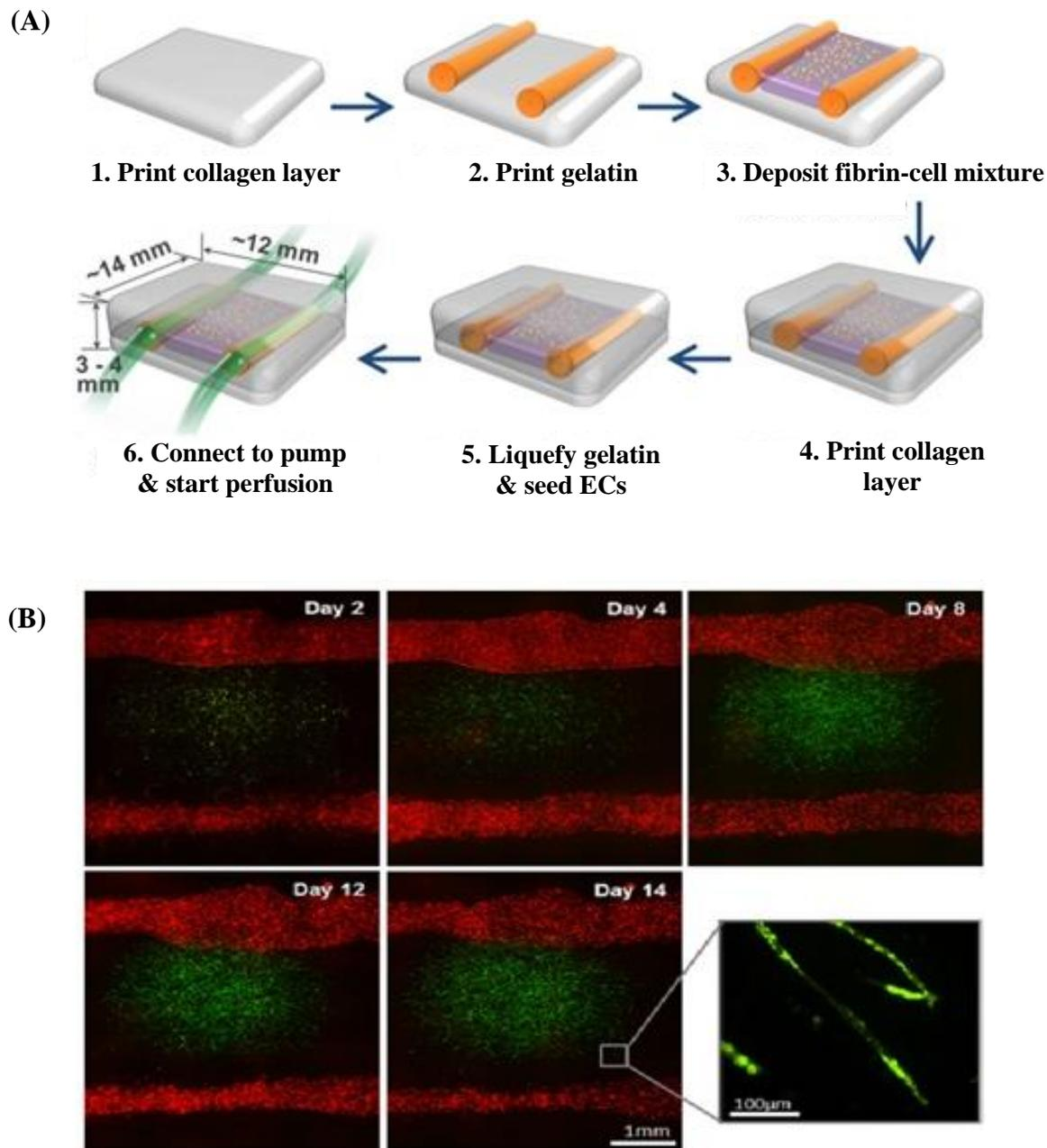
**Fig. 2.** Extrusion printing method. (A) A schematic picture of two large channel structures and deposition of fibrin and cell, which were developed using the 3D bioprinter. (B) Florescent microscopic images of two large channels, and the mixture of fibrin cell placed between channels. Green dots show green fluorescent protein-ECs that were cultured within fibrin, and red dots indicate red fluorescent protein-ECs that were seeded on the two large channels<sup>[55]</sup>.
