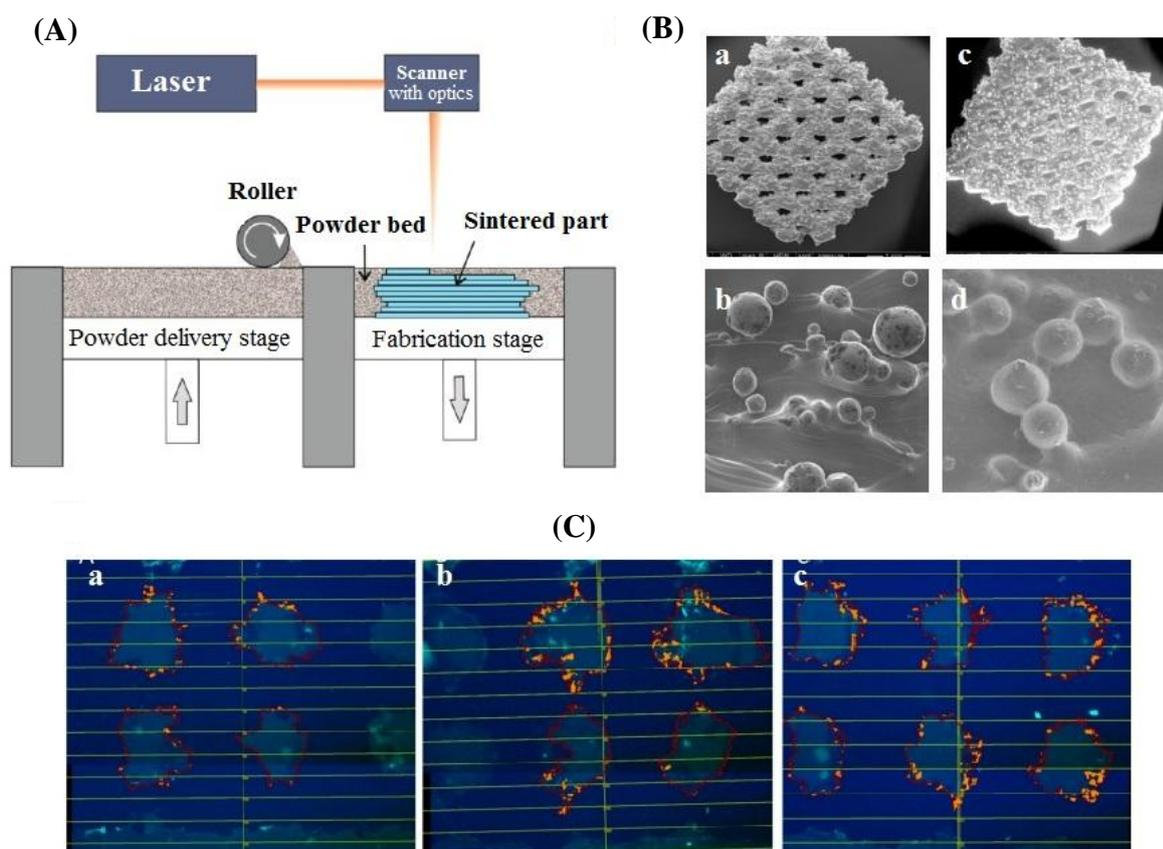
**Fig. 3.** Selective laser sintering (SLS) methods. (A) A schematic picture of a SLS printer; (B) environmental scanning electron microscopy photos of three different samples, non-coated (a and b) and polycaprolactone-coated (c and d); (C) Wimasis image analysis of titanium implant's crosssection with green fluorescent protein-osteoblasts seeded in different times: (a) one day, (b) three days, and (c) seven days.
