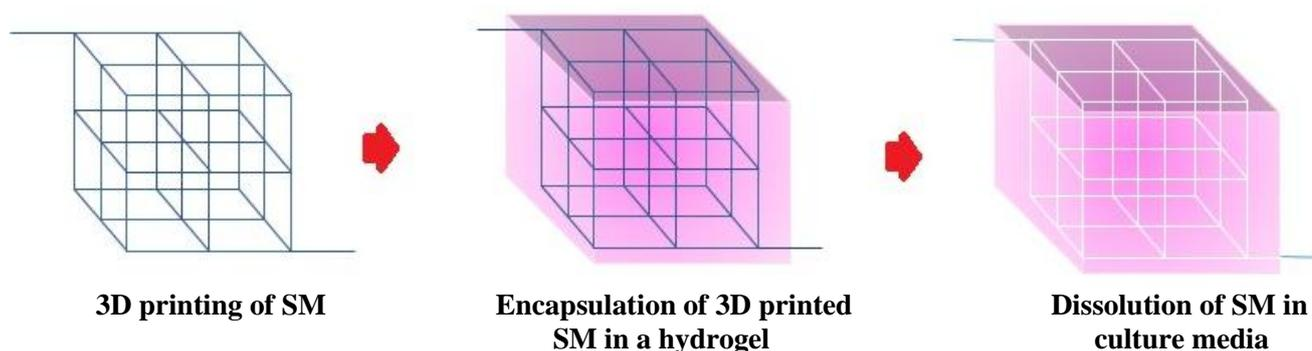
**Fig. 5.** The process of the microchannel formation inside the gel using the 3D printing of sacrificial materials (SM). At first, a computer-based plan of a SM is fabricated using the 3D printing. Then this 3D construct was immersed in a solution of an appropriate biomaterial and certain cells. After gelation of the biomaterial, the 3D constructs were immersed in culture media, which flows inside the channel, dissolves SM, and creates microchannel within the scaffolds.
