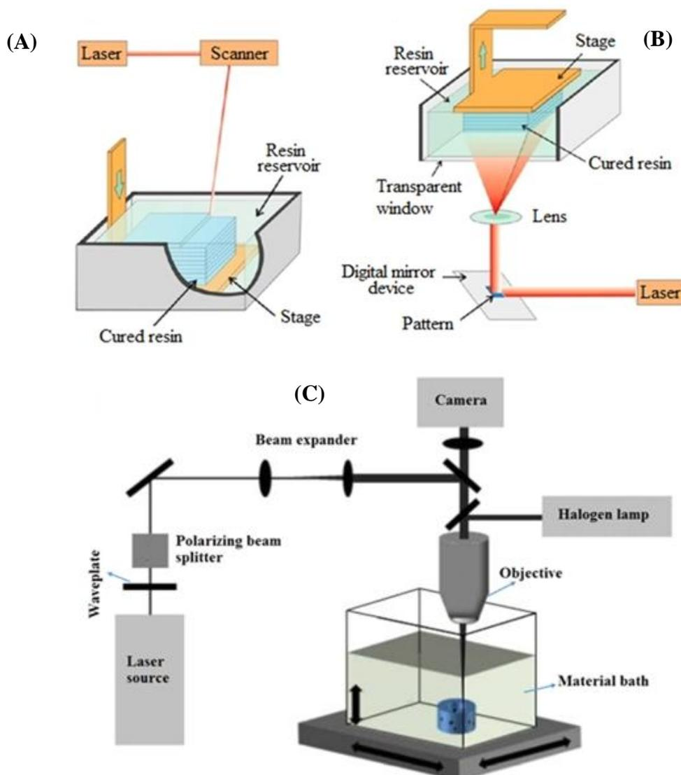
**Fig. 4.** Stereolithography method of printing. (A) direct and (B) indirect or mask-based stereolithography. (C) An illustration of stereolithography to fabricate vessels in Huber *et al.*'s<sup>[71]</sup> study. A laser beam was polarized, expanded and then directed through a microscope objective.
