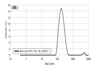
Fig. 3. Dynamic light scattering analysis of NMB OMVs. (A) Zeta potential distribution of NMB OMVs; (B) Size distribution by intensity or zeta average and PDI.
