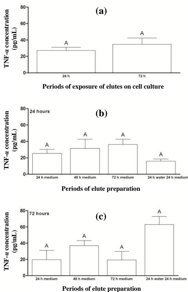
**Fig. 3.** Concentration of TNF-  $\alpha$  (a) after the exposure of acrylic resin eluates to cell cultures for periods of 24 and 72 hours and for preparing eluates prior to their exposure to cell cultures for (b) 24 h and (c) 72 h. The results show mean  $\pm$  standard error of TNF- $\alpha$  concentration (pg/mL). Different capital letters for each chart indicate statistical difference ( $p < 0.05$ ) between the groups.
