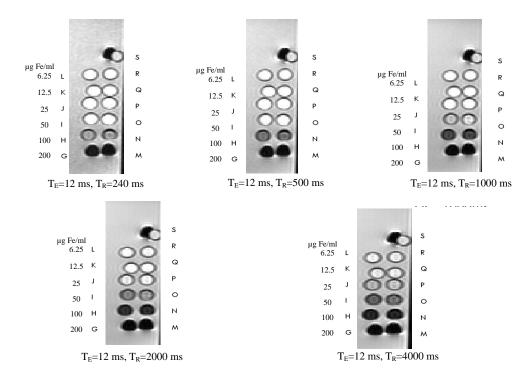
**Fig. 5.**  $T_1$ -weighted spin-echo image of Nanomag®-D-SPIO and SPIONs-C595 in 1 ml.  $T_R$ =250, 500, 1000, 2000, and 4000 ms,  $T_E$ =12 ms. M, N, O, P, Q, and R are the SPIONs-C595 with different concentrations of 200, 100, 50, 25, 12.5, 6.25  $\mu$ g Fe/ml. However, G, H, I, J, K, and L are the Nanomag®-D-SPIO with the same concentrations as SPIONs-C595, respectively. S is the distilled water for control.
