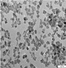
**Fig. 1.** Transmission electron microscopy images of (A) Nanomag®-D-SPIO and (B) SPIONs-C595. Monoclonal antibody binding caused a significant reduction in particle agglomeration.
