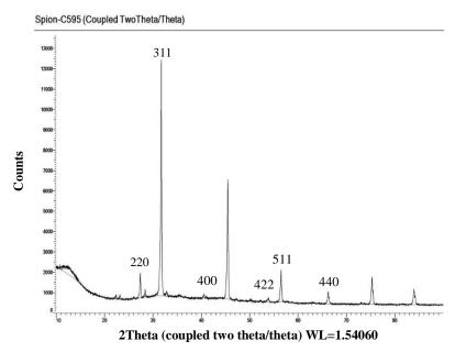
Fig. 3. X-ray diffraction pattern of SPIONs-C595. The peaks correspond for both  $Fe_2O_3$  and  $Fe_3O_4$  are the same as compared with JCPDS data (PDF number). PDF number is the powder diffraction file. Fe3O4 crystal of JCPDS data (PDF 01-078-6086), Fe2O3 crystal of JCPDS data (PDF 09-054-0489).
