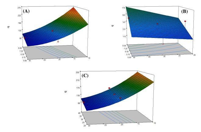
**Fig. 3.** Response surface plot of different factors interactions. (A) The interactive effect of the biomass dosage and pH at constant temperature 30°C on metal uptake (q); (B) the effect of temperature and pH at constant biomass dosage of 2 mg/mL on the metal uptake (q); (C) the effect of temperature and biomass dosage at constant pH of 6.5 on metal uptake (q).
