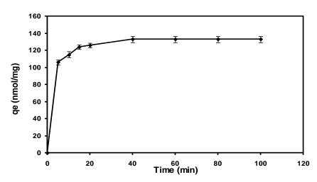
**Fig. 1.** Effect of contact time on the biosorption capacity of Cd (II) (q<sub>e</sub>) by *E. coli* E. [Cd (II)] concentration, 20 mg/L; biomass dosage, 1 mg/mL Tris-HCl, pH 6.5, 30°C, 100 rpm).
