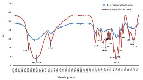
Fig. 4. The FTIR spectra of our developed bioadsorbent in the absence and presence of cadmium.
