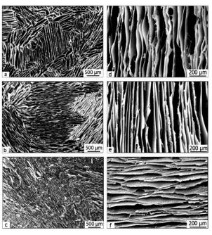
**Fig. 2.** Scanning electron micrograph of the scaffolds in both parallel and perpendicular to solidification direction. (a) R0.5G0.8, perpendicular; (b) R1G0.8, perpendicular; (c) R2G0.8 perpendicular, (d) R0.5G0.8 parallel; (e) R1G0.8 parallel; (f) R2G0.8, parallel. The uniform morphology of the pores is created by constant freeze-casting rate at -196°C.
