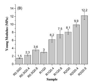
**Fig. 4.** Mechanical properties. (A) Scaffolds tensile strength (B) Young's modulus (n=3). Tensile strength and elastic modulus were under the influence of the both glutaraldehyde content and freezing rate.
