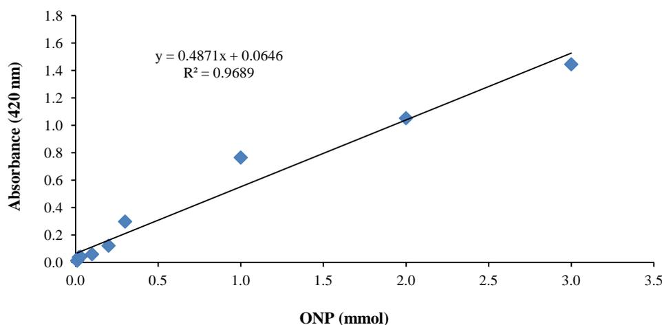
**Fig 1.** Standard calibration curve of o-nitrophenol (ONP)
