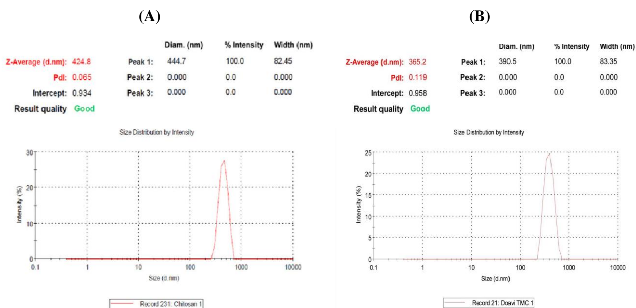
Fig. 1. The nanoparticles size distribution measured by Zetasizer. A) Electrospayed chitosan nanoparticles containing rEIT (about 424/8 nm); B) Electrospayed TMC nanoparticles containing rEIT (about 365/2 nm).
