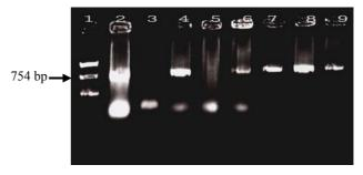
**Fig. 3**. Clones analysis with Direct PCR. Lane 1, pUC18/Taq1 marker; Lane 2, posetive control; Lane 3, negetive control; Lane 5, PET without insert; Lanes 4 and 6-9 clones.
