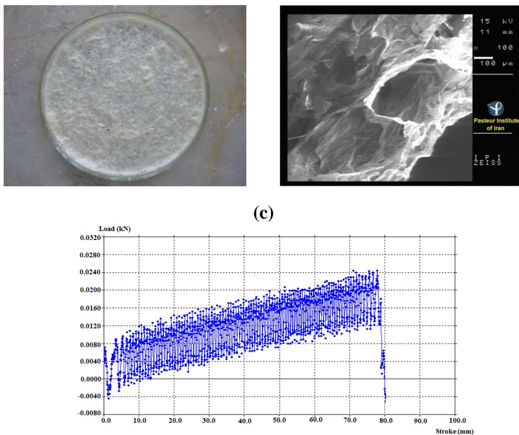
**Fig. 3.** Collagen-chitosan evaluation fabricated by freeze-gelation method. (a) direct observation; (b) scanning electron microscopy and (c) tensile test.
