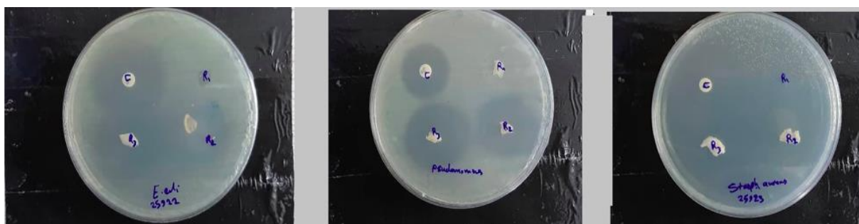
Fig. 6. Inhibition zone of S. aureus , E. coli , and P. aeruginosa around films after 24 h of incubation in a Muller Hinton agar plate. C, positive control (ciprofloxacin); R 1 : SF; R 2 : SF/Th; R 3 : SF/N/Th.
