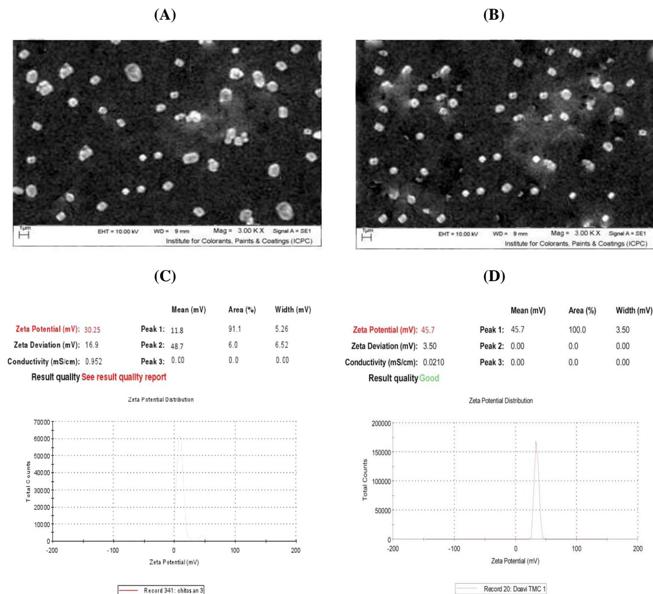
**Fig. 2.** SEM images of electrospayed nanoparticles and zeta potentials. A) SEM images of electrospayed chitosan nanoparticles containing rEIT; B) TMC nanoparticles containing rEIT; C) Zeta potential of electrospayed chitosan nanoparticles containing rEIT (about +30/25 mV); D) electrospayed TMC nanoparticles containing rEIT (about +45/7 mV).
