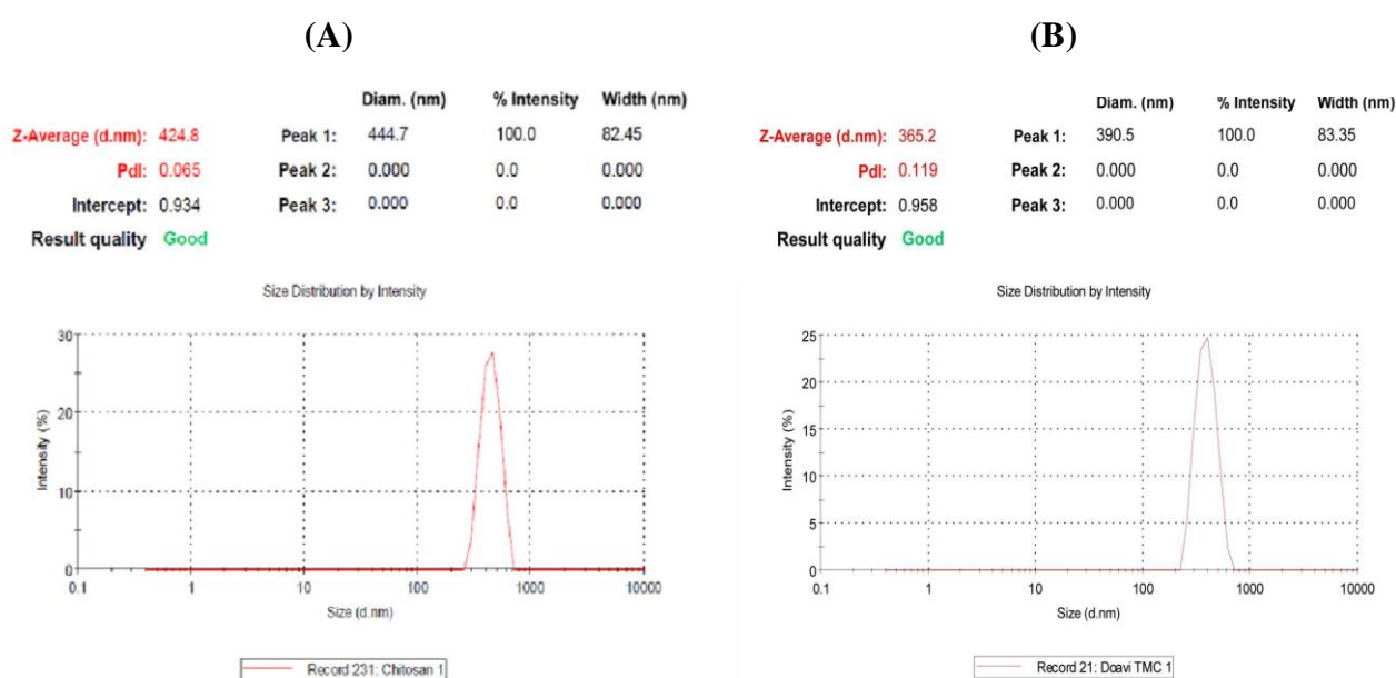
Fig. 1. The nanoparticles size distribution measured by Zetasizer. A) Electro sprayed chitosan nanoparticles containing rEIT (about 424.8 nm); B) Electro sprayed TMC nanoparticles containing rEIT (about 365.2 nm).
