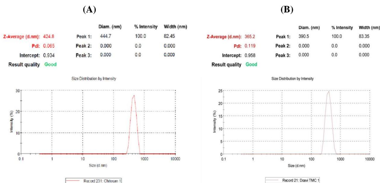
**Fig. 1.** The nanoparticles size distribution measured by Zetasizer. A) Electrospayed chitosan nanoparticles containing rEIT (about 424/8 nm); B) Electrospayed TMC nanoparticles containing rEIT (about 365/2 nm).
